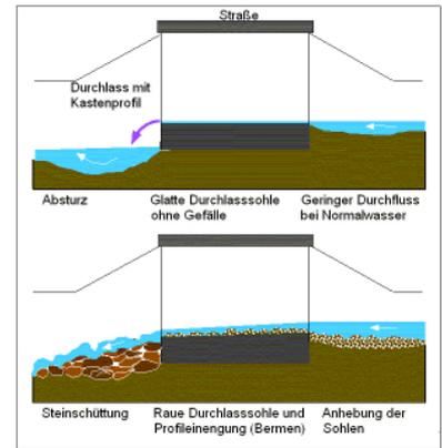
(7) Bio-permeability under a bridge (Schema)
