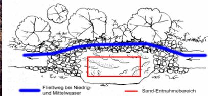
(6) Schematic of a sand trap
